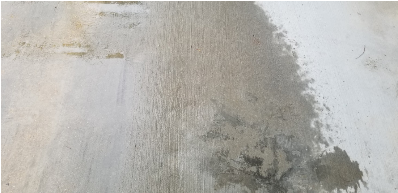
Figure 5-13: Concrete Surface with Three Levels of Wetness: Dry, Wet, and Puddled Water.
