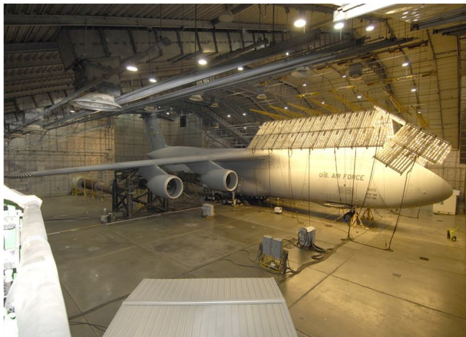
Figure 8-14: View of the Largest Indoor Weather Testing Facility in the World McKinley Climatic Lab in Florida, 76.8 x 61.2 x 21m 3 [5].
