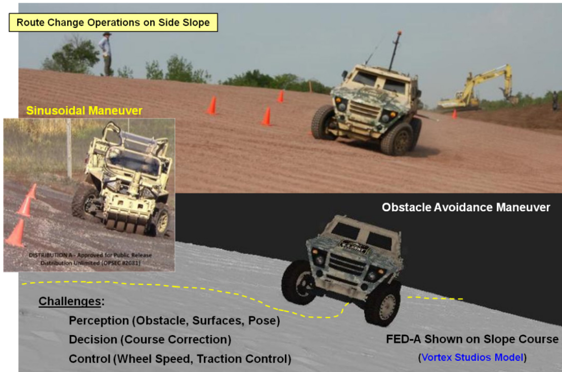
Figure 8-17: Expanded Mobility Event (Unpaved Side Slope Object Avoidance).
