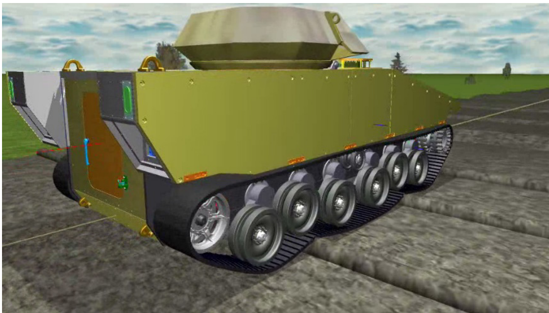
Figure 6-28: Tracked Vehicle w/ a Belt Track Simulated Using the DIS Code [66] Going Over Semi-Circular Bumps [61].
