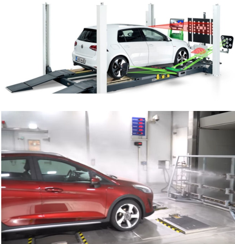
Figure 8-11: Sensor Validation Using Test Rig in Environmental Chamber [4].
